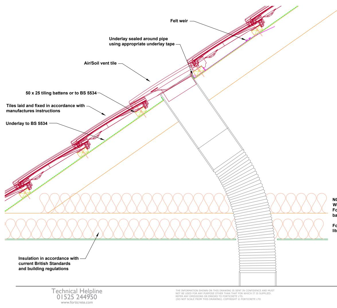
NOTES: When using a vapour permeable (LR) underlay, Forticrete in line with BS5250 recommend that the batten cavity is ventilated from eave to ridge.
